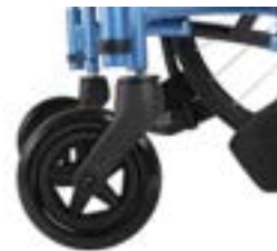
Figure 4 Correct caster position to the front
