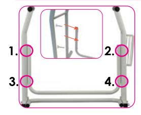
IMPORTANT: Screws MUST be attached in the exact order stated in # 1 and # 2 of Assembly Instructions
